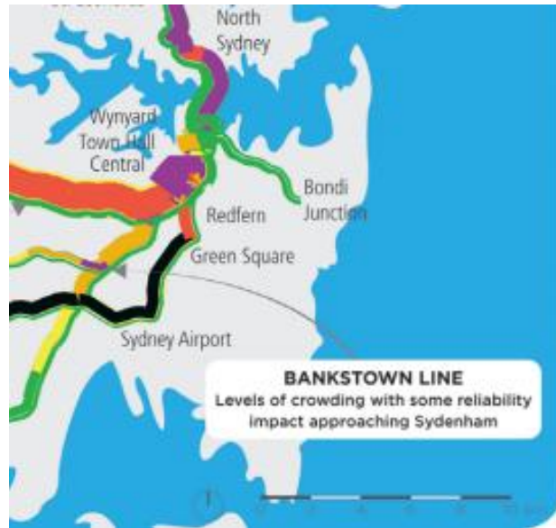
FIGURE 13. RAIL NETWORK PERFORMANCE (REPRESENTED BY VOLUME- CAPACITY RATIO), AM PEAK, 2031 'DO NOTHING' SCENARIO
